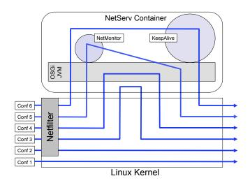
Figure 11: Test configurations 1 to 6.
