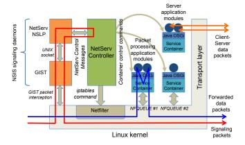
Figure 2: NetServ node prototype.
