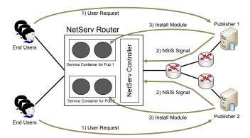
Figure 1: Deploying modules on a NetServ node.
