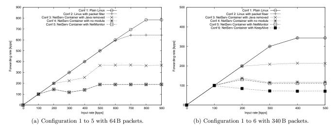
Figure 12: Forwarding rates of the router with different configurations.
