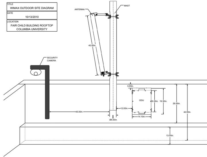
Figure 1: Diagram for WiMAX deployment (outdoor on Fairchild rooftop)
