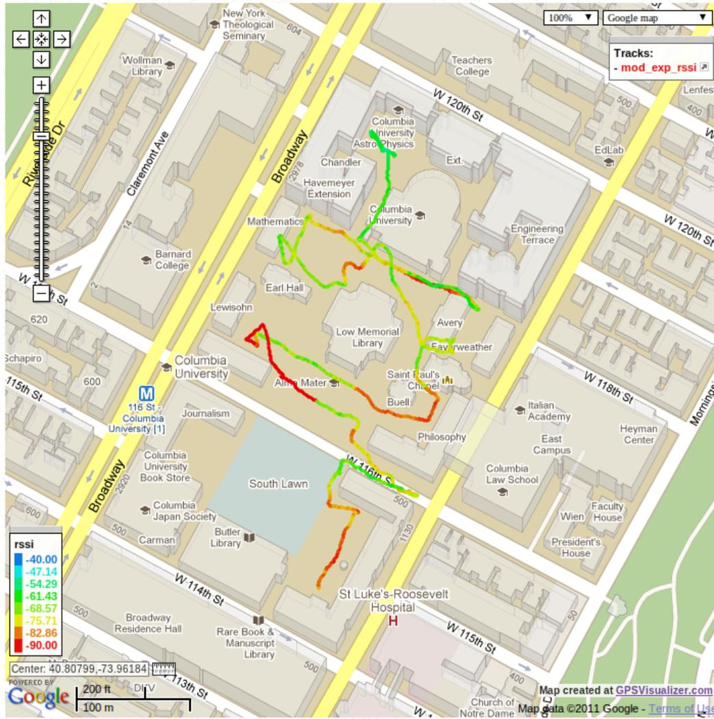
Figure 21: Measured WiMAX RSSI and location mapping with GPSVisualizer
