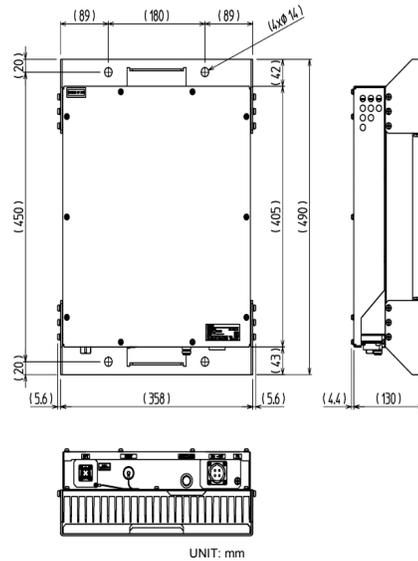
Figure 2: Diagram for WiMAX ODU
