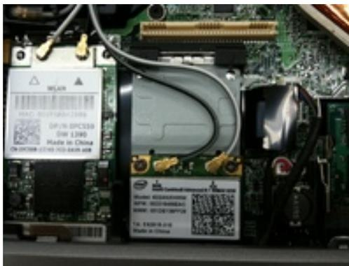
Figure 12: Installed NIC with bracket
