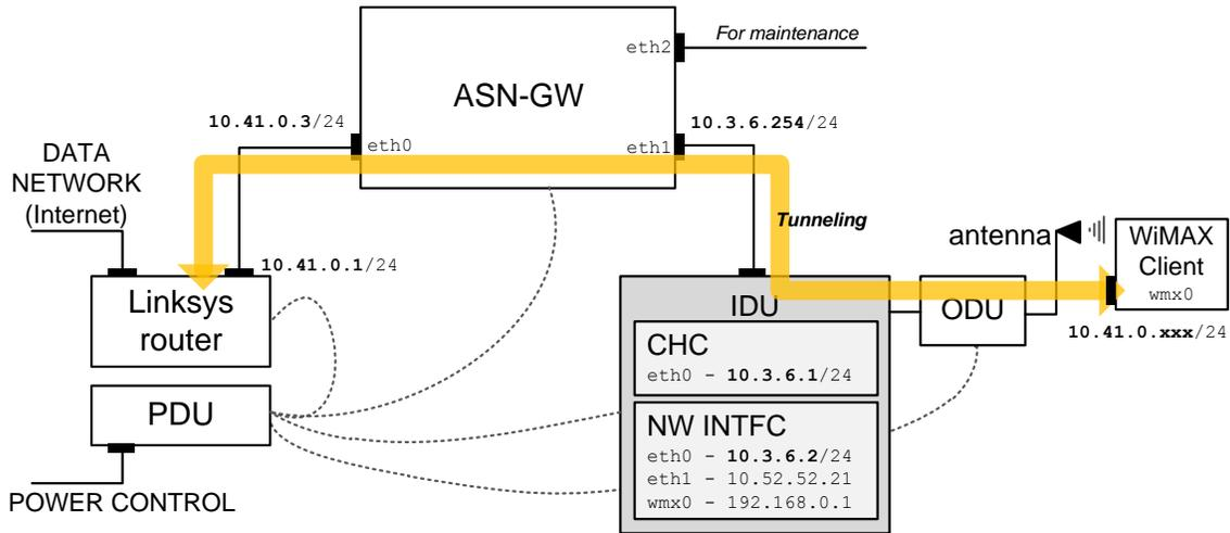
Figure 9: IP allocation for deployment: A WiMAX client obtains an IP address provided by DHCP on Linksys Router and makes a tunnel over the ASN-GW and WiMAX base station
