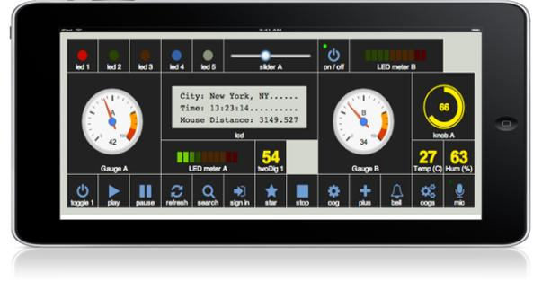
Figure 5. An example of a control panel showing an assorted collection of port view widgets. Each widget is connected to a virtual port and either controls the port or displays its value. The application provides a drag and drop UI to create such panels. The panel is running in the Chrome browser on a mobile device (tablet).
